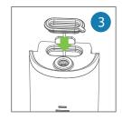
Fill the tank with the water and put the plug.
