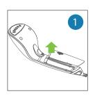
Remove the water tank by pulling it down.
