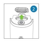
Remove the silicone plug from the water tank.
